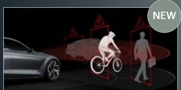
Forward Collision Avoidance Assist (FCA) - Car/Pedestrian/Cyclist with Junction Turning
